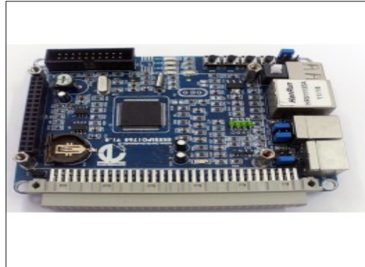
Fig. 6. LPC 1768 board designed for on-board
